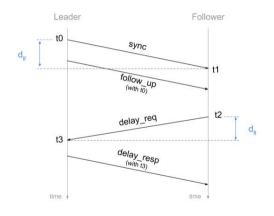
The trip time include the transmit time and the delta between the two clocks:
