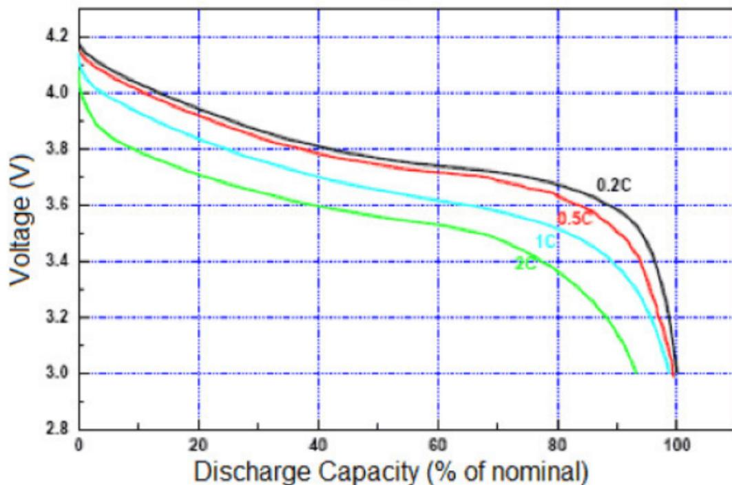
Discharge: 3.0V cutoff at room temperature.
