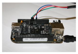
Once the USB to Serial connector is plugged in, a new serial port should appear: /dev/ttyUSB0. You can also see this device appear by looking at the output of dmesg.
