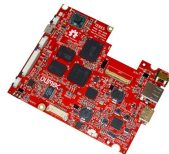
Olimex Open hardware ARM laptop main board
