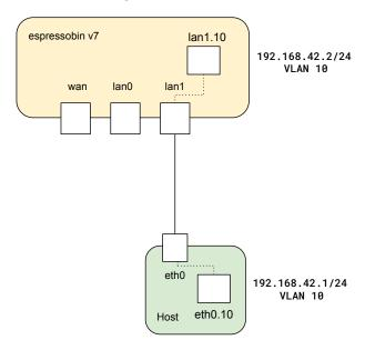
We'll use a dedicated netdevice for the VLAN we want to create. We will use VLAN id 10, which is arbitrary here. We assign an IP address to the vlan interface, and set it as admin-up:
