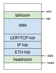
Our custom tag needs to be inserted **before** the Ethernet header, that is, between the Layer 3 header and the Layer 2 header. We therefore need to move the Ethernet header down into the headroom of the SKB.
