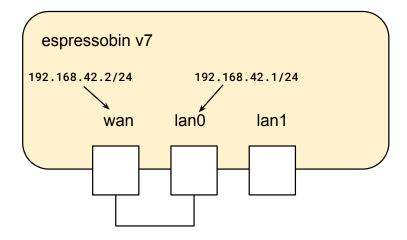
Connect wan and lan0 together with one of the provided Ethernet cables, and configure both interfaces with the ip command, using the addresses indicated in the above schematic.
