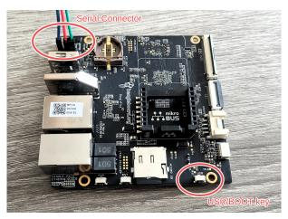
If the USR key is released, then the SoC will try to find a bootloader into eMMC memory. If the USR key is pressed, then it will try to find a bootloader on the microSD.
